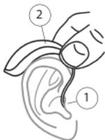
1. Insert the ear-set into the ear while holding the lower part of the earwire. Pulling the outer ear upwards and backwards at the same time can be helpful.
